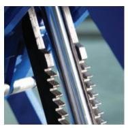
24 lock positions feature a negative rake tooth design. Locks ratchet over each other then interlock when lift is lowered to locks.
